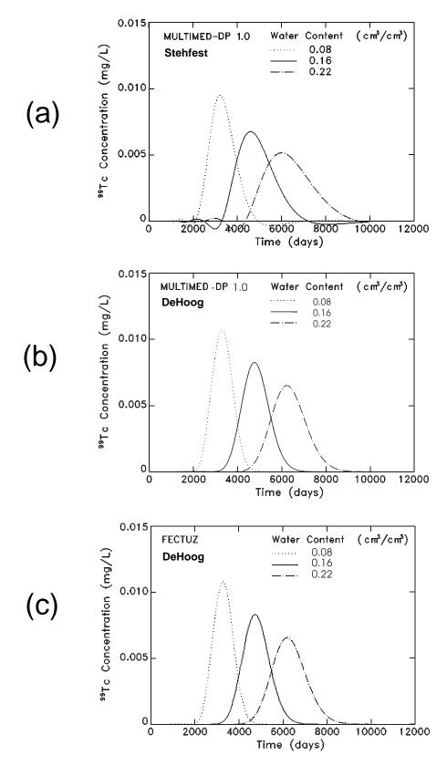
**Figure 7-26.** Sensitivity of <sup>99</sup>Tc BTCs at 6m depth to water content, where (a) uses Stehfest Algorithm of MULTIMED-DP 1.0, (b) uses DeHoog Algorithm of MULTIMED-DP 1.0, and (c) uses DeHoog Algorithm of FECTUZ Code.
