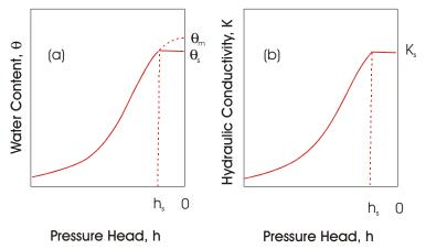
**Figure A-1.** Schematics of the soil-water retention curve (a) and the hydraulic conductivity function (b) for the VC-Model (from Simunek et al., 1998).
