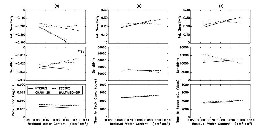
**Figure 7-22.** Sensitivity and relative sensitivity of (a) peak concentration at the depth of 6m, (b) time to reach peak concentration at the depth of 6m, and (c) time to exceed MCL at the receptor well to the residual water content using the MULTIMED-DP 1.0, FECTUZ, CHAIN 2D, and HYDRUS Models.
