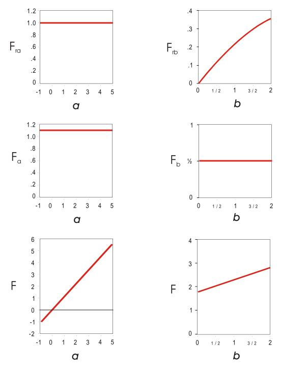
**Figure 4-2.** Sensitivities and relative sensitivities of F with respect to a and b, with reference to the base case in Equation (4-10).
