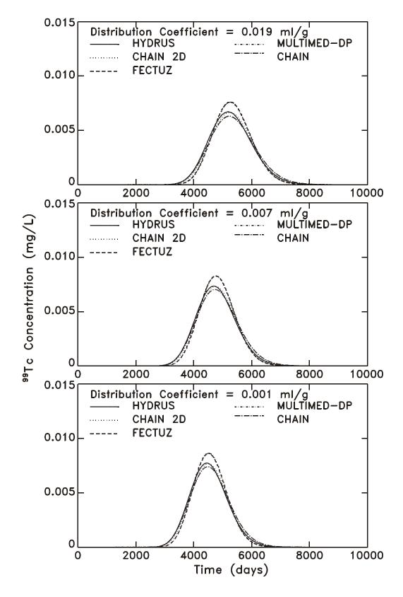
**Figure 7-1.** Sensitivity of  $^{99}$ Tc breakthrough (through the 6m layer) to the distribution coefficient using the CHAIN, MULTIMED-DP 1.0, FECTUZ, CHAIN 2D, HYDRUS Models, where  $K_d = 0.019$  ml/g, and 0.001 ml/g.
