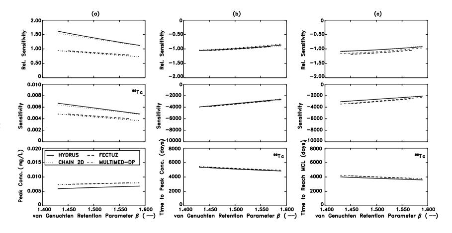
Figure 7-24. Sensitivity and relative sensitivity of (a) peak concentration at the depth of 6m, (b) time to reach peak concentration at the depth of 6m, and (c) time to exceed MCL at the receptor well to the van Genuchten retention parameter β using the MULTIMED-DP 1.0, FECTUZ, CHAIN 2D, and HYDRUS Models.
