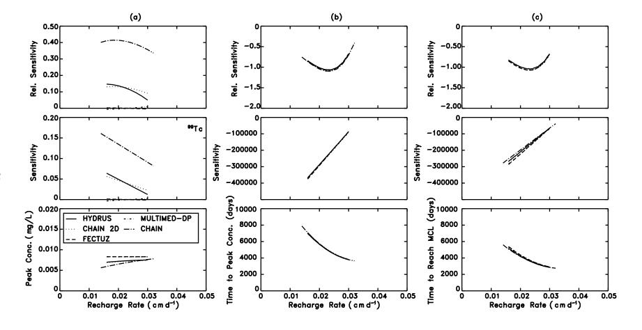
Figure 7-14. Sensitivity and relative sensitivity of (a) peak concentration at the depth of 6m, (b) time to reach peak concentration at the depth of 6m, and (c) time to exceed MCL at the receptor well to the recharge rate using the CHAIN, MULTIMED-DP 1.0, FECTUZ, CHAIN 2D and HYDRUS Models.
