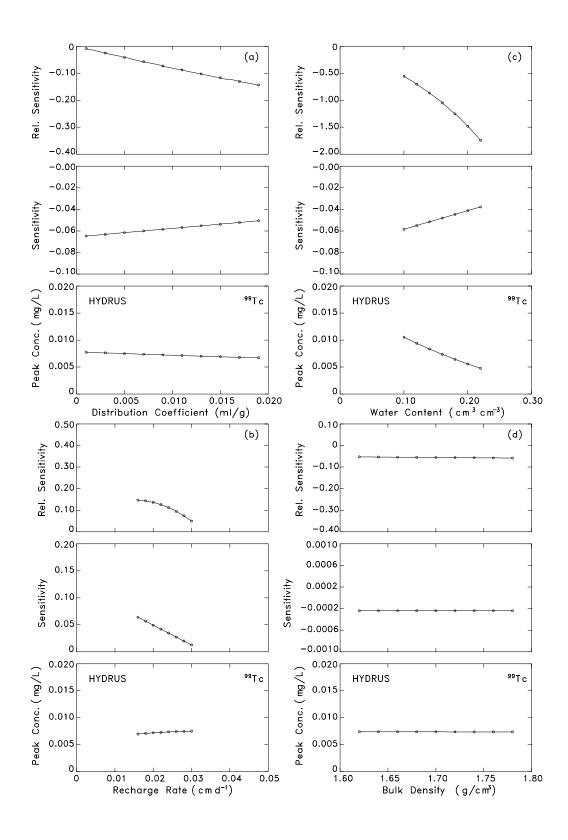
**Figure 6-2.** Sensitivity and relative sensitivity of peak concentrations at the depth of 6m to the system parameters using the HYDRUS Model: (a) distribution coefficient, (b) recharge rate, (c) water content, (d) bulk density.
