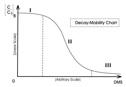
**Figure I-1.** The normalized concentration of a radionuclide at the bottom of a soil column (the source being at the top of the column) versus a hypothetical decay-mobility scale (DMS), where I represents highly mobile, long-lived species, III represents highly immobile, short-lived species, and II represents species with intermediate mobilities and half-lives.
