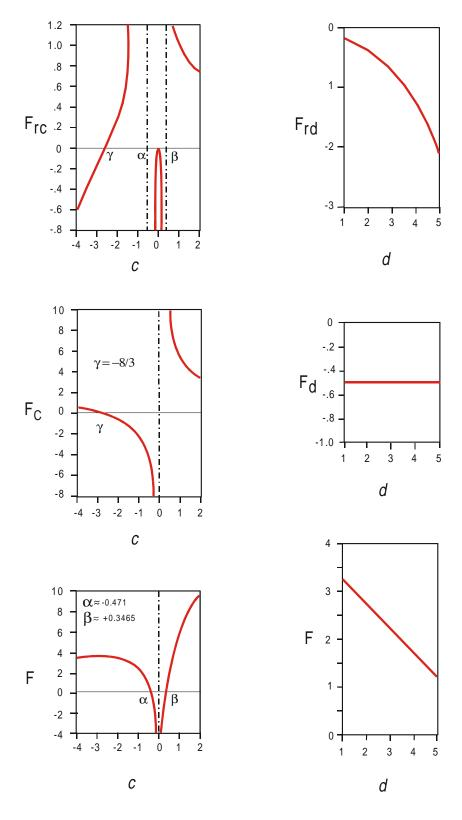
**Figure 4-3.** Sensitivities and relative sensitivities of F with respect to c and d, with reference to the base case in Equation (4-10).
