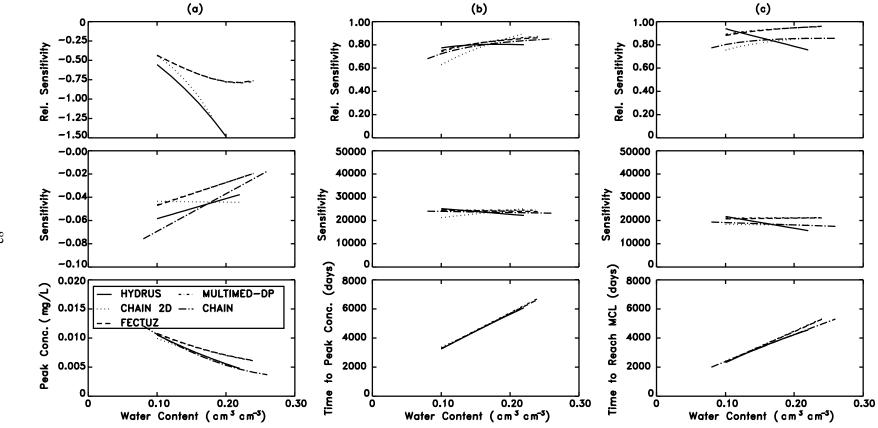
Figure 7-15. Sensitivity and relative sensitivity of (a) peak concentration at the depth of 6m, (b) time to reach peak concentration at the depth of 6m, and (c) time to exceed MCL at the receptor well to the water content using the CHAIN, MULTIMED-DP 1.0, FECTUZ, CHAIN 2D and HYDRUS Models.
