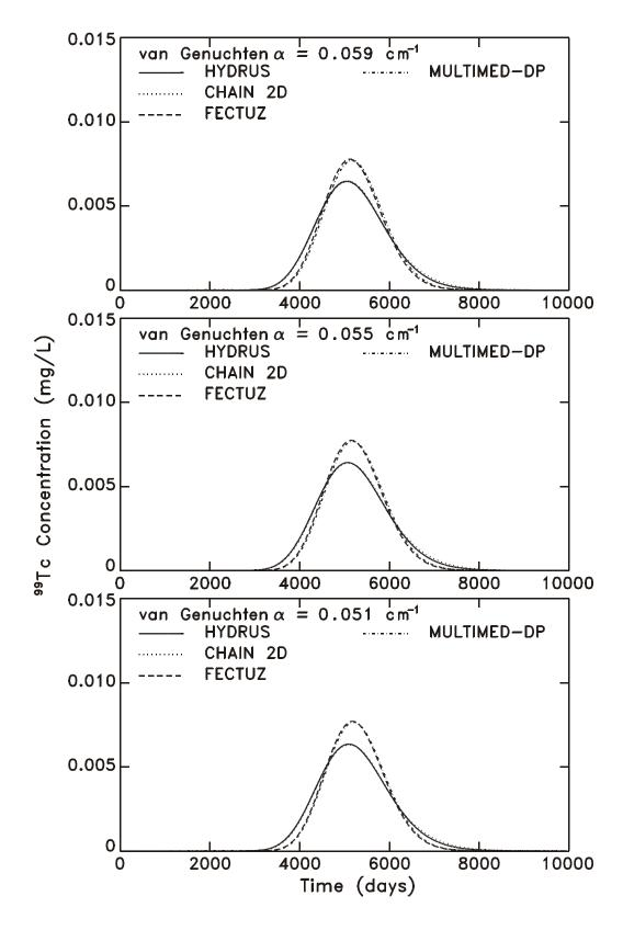
Figure 7-11. Sensitivity of  $^{99}$ Tc breakthrough (through the 6m layer) to the van Genuchten retention parameter  $\alpha$  using the MULTIMED-DP 1.0, FECTUZ, CHAIN 2D and HYDRUS Models, where  $\alpha = 0.059 cm^{-1}$ ,  $0.055 \ cm^{-1}$ , and  $0.051 \ cm^{-1}$ .
