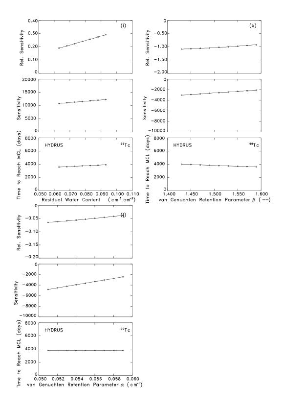
Figure 6-4. Sensitivity and relative sensitivity of time to exceed MCL to the system parameters using the HYDRUS Model: (i) residual water content, (j) van Genuchten retention parameter  $\alpha$ , (k) van Genuchten retention parameter  $\beta$ .
