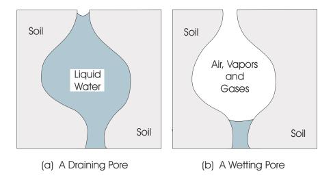
Figure C-5. The "ink bottle" effect demonstrating that draining/drying soils under the influence of capillary forces retain more water at a given soil-water pressure than a wetting soil at the same water pressure (reprinted from *Unsaturated Zone Hydrology*, 1994, by Gary L. Guymon, with permission of Pearson Education, Inc., Upper Saddle River, NJ).
