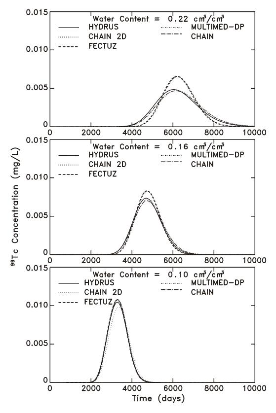
**Figure 7-3.** Sensitivity of <sup>99</sup>Tc breakthrough (through the 6m layer) to the water content using the CHAIN, MULTIMED-DP 1.0, FECTUZ, CHAIN 2D, and HYDRUS Models, where  $\theta = 0.22$  cm<sup>3</sup>/cm<sup>3</sup>, 0.16 cm<sup>3</sup>/cm<sup>3</sup>, and 0.10 cm<sup>3</sup>/cm<sup>3</sup>.
