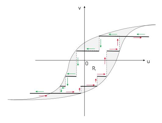
**Figure C-3b.** An approximation to a continuous hysteresis loop by a linear combination of a finite family of delayed relays. The quantity  $R_f$  is the region inside the discontinuous loop formed by the finite family of relays (reprinted from *Differential Models of Hysteresis*, 1994, by Augusto Visintin, with permission of Springer-Verlag, GmbH & Co. KG, Heidelberg, Germany).
