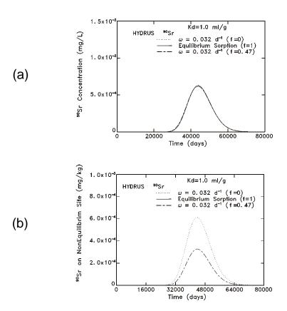
**Figure H-1.** The c- and s distribution of Equations (H-1) and (H-2) for  ${}^{90}$ Sr for  $(\omega, f) = (0, 1)$ ,  $(0.032 \, d^{-1}, 0.47)$ ,  $(0.032 \, d^{-1}, 0)$ . Distributions were derived by the HYDRUS Code, (a) gives the concentration in solution and (b) gives the concentration on the soil matrix.
