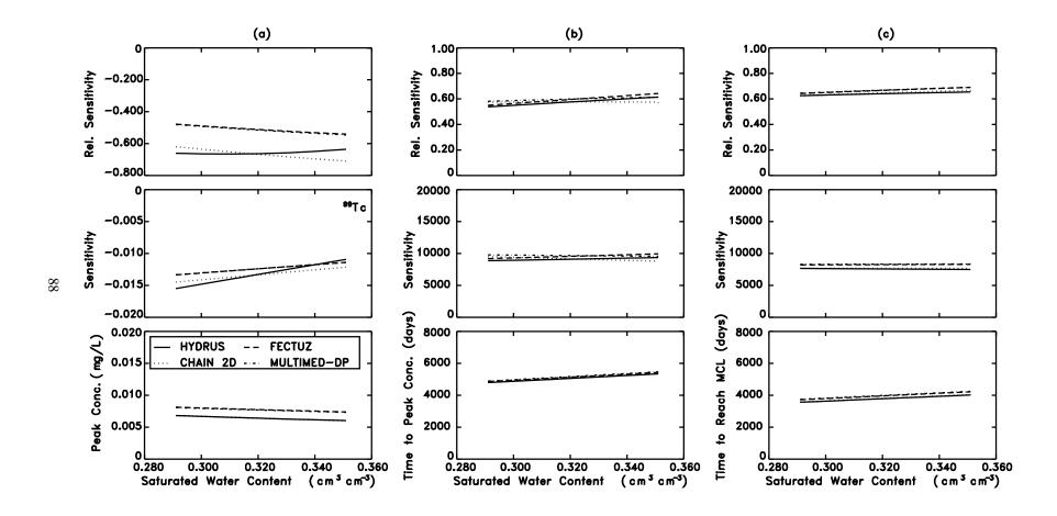
Figure 7-21. Sensitivity and relative sensitivity of (a) peak concentration at the depth of 6m, (b) time to reach peak concentration at the depth of 6m, and (c) time to exceed MCL at the receptor well to the saturated water content using the MULTIMED-DP 1.0, FECTUZ, CHAIN 2D, and HYDRUS Models.
