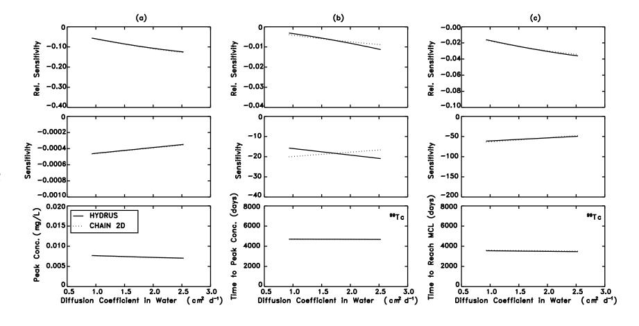
**Figure 7-19.** Sensitivity and relative sensitivity of (a) peak concentration at the depth of 6m, (b) time to reach peak concentration at the depth of 6m, and (c) time to exceed MCL at the receptor well to the diffusion coefficient in water using the CHAIN 2D and HYDRUS Models.
