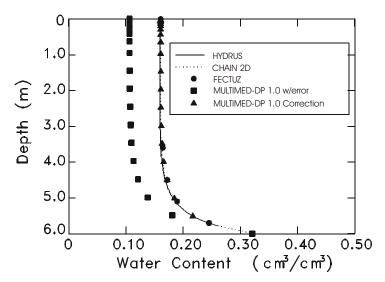
Figure 7-25. Water content distributions predicted by the HYDRUS, CHAIN 2D, FECTUZ, and MULTIMED-DP 1.0 models. Note that the water contents (■) obtained from the originally distributed MULTIMED-DP 1.0 code are in error. The corrected code gives a consistent water content distribution (▲) with the other three models.
