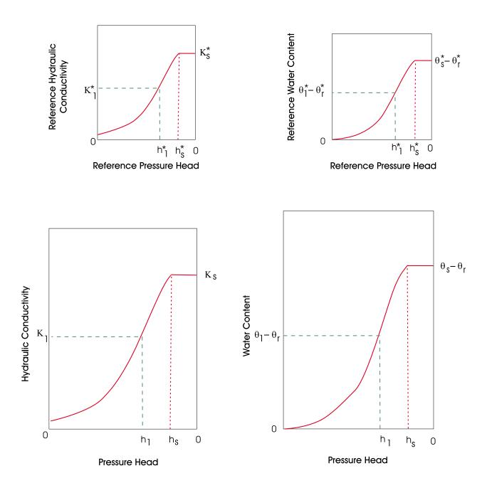
$\begin{array}{ll} \textbf{Figure 2-2.} & \text{An example of soil structure scaling for scale factors } (\alpha_h,\alpha_\theta,\,\alpha_k) = (3/2,\,2,\,7/4). & \text{The ratios } h_s/h_s^{\ *} = h_1/h_1^{\ *} = 3/2,\, (\theta_s\text{-}\ \theta_r) \div (\theta_s^{\ *}\text{-}\ \theta_r^{\ *}) = (\theta_1\text{-}\ \theta_r) \div (\theta_1^{\ *}\text{-}\ \theta_r^{\ *}) = 2,\, \text{and } K_1/K_1^{\ *} = K_s/K_s^{\ *} = 7/4. \\ \end{array}$
