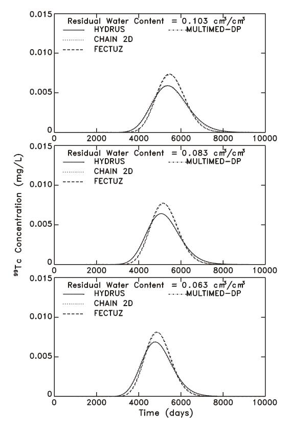
Figure 7-10. Sensitivity of  $^{99}\text{Tc}$  breakthrough (through the 6m layer) to the residual water content using the MULTIMED-DP 1.0, FECTUZ, CHAIN 2D and HYDRUS Models, where  $\theta_r = 0.103 \text{ cm}^3/\text{cm}^3$ ,  $0.083 \text{ cm}^3/\text{cm}^3$ , and  $0.063 \text{ cm}^3/\text{cm}^3$ .
