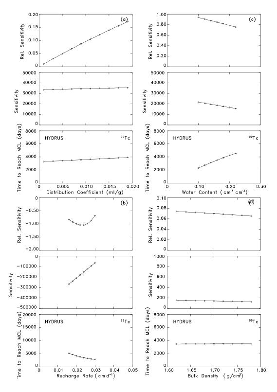
**Figure 6-4.** Sensitivity and relative sensitivity of time to exceed MCL to the system parameters using the HYDRUS Model: (a) distribution coefficient, (b) recharge rate, (c) water content, (d) bulk density.
