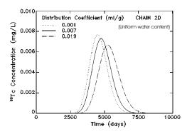
**Figure E-3.** Sensitivity of <sup>99</sup>Tc breakthrough (through the 6 m layer) to the distribution coefficient using the CHAIN 2D Model, for a nonuniform water content (top) and for a uniform water content (bottom).
