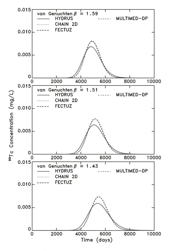
Figure 7-12. Sensitivity of  $^{99}$ Tc breakthrough (through the 6m layer) to the van Genuchten retention parameter  $\beta$  using the MULTIMED-DP 1.0, FECTUZ, CHAIN 2D and HYDRUS Models, where  $\beta$  = 1.59, 1.51, and 1.43.
