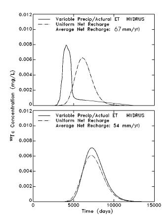
Figure F-4. Comparison of predicted <sup>99</sup>Tc breakthrough curves (through the 6 m layer) using the variable precipitation/actual ET versus uniform recharge rate in the HYDRUS Model. Average recharge rate is calculated as the mean net amount of precipitation and actual ET from 0 to 12,000 days. The net recharge varies between the two sets of curves due to the root-uptake scenario, (h<sub>1</sub>,h<sub>2</sub>,h<sub>3</sub>).
