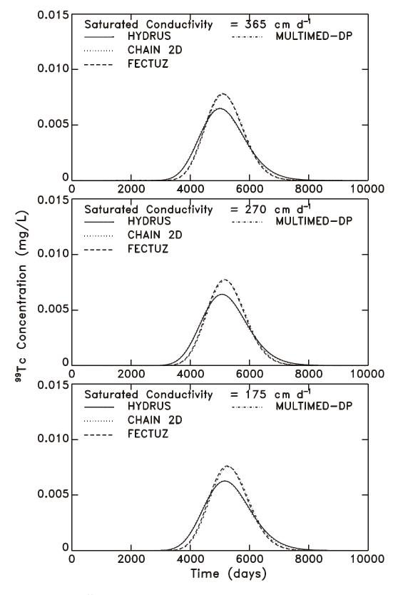
**Figure 7-8.** Sensitivity of  $^{99}$ Tc breakthrough (through the 6m layer) to the saturated conductivity using the MULTIMED-DP 1.0, FECTUZ, CHAIN 2D and HYDRUS Models, where  $K_s = 365$  cm/d, 270 cm/d, and 175 cm/d.
