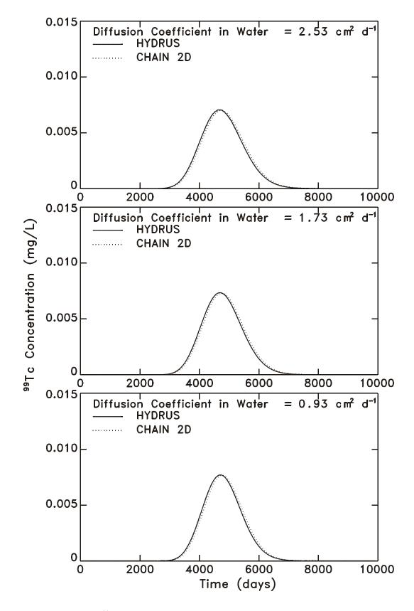
Figure 7-7. Sensitivity of  $^{99}$ Tc breakthrough (through the 6m layer) to the diffusion coefficient in water using the CHAIN 2D and HYDRUS Models, where  $D_w = 2.53 \text{ cm}^2/\text{d}$ ,  $1.73 \text{ cm}^2/\text{d}$ , and  $0.93 \text{ cm}^2/\text{d}$ .
