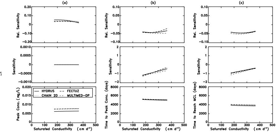
Figure 7-20. Sensitivity and relative sensitivity of (a) peak concentration at the depth of 6m, (b) time to reach peak concentration at the depth of 6m, and (c) time to exceed MCL at the receptor well to the saturated conductivity using the MULTIMED-DP 1.0, FECTUZ, CHAIN 2D, and HYDRUS Models.
