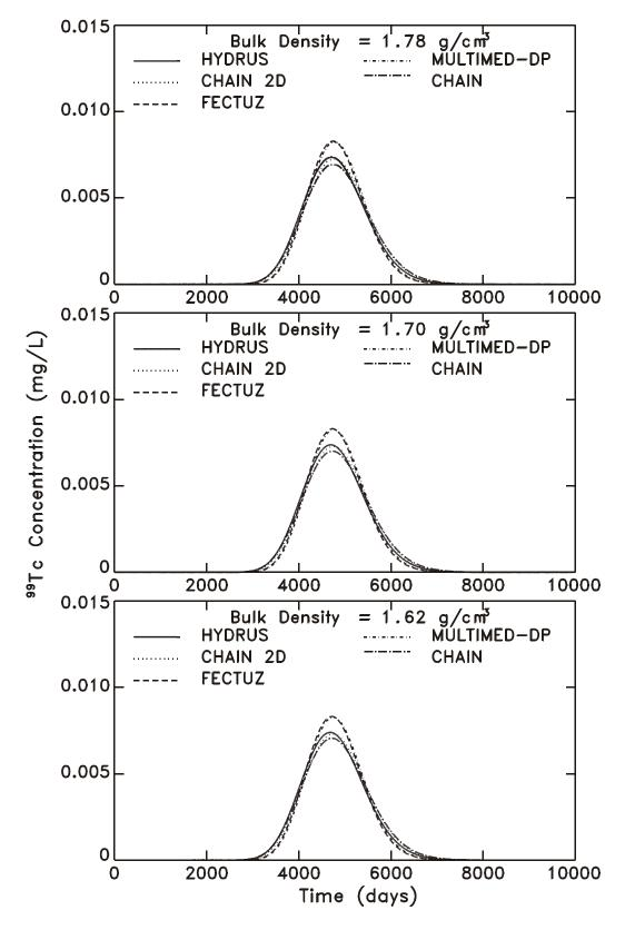
**Figure 7-4.** Sensitivity of <sup>99</sup>Tc breakthrough (through the 6m layer) to the bulk density using the CHAIN, MULTIMED-DP 1.0, FECTUZ, CHAIN 2D, and HYDRUS Models, where  $\rho = 1.78$  g/cm<sup>3</sup>, 1.70 g/cm<sup>3</sup>, and 1.62 g/cm<sup>3</sup>.
