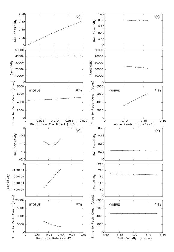
**Figure 6-3.** Sensitivity and relative sensitivity of time to reach peak concentrations at the depth of 6m to the system parameters using the HYDRUS Model: (a) distribution coefficient, (b) recharge rate, (c) water content, (d) bulk density.
