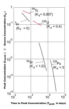
**Figure I-4.**  $C_{peak} \div C_o$  versus  $T_{peak}$  in days for five radionuclides, showing the effects of various  $K_d$  values and various decay rates, where the time intervals of the curve segments are determined by the range of discharge rates for the 6 m soil column.
