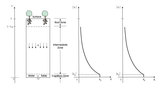
**Figure 2-1.** Schematic of an unsaturated soil column, soil-water retention curve, and hydraulic conductivity function, where subscript "s" indicates saturated conditions.
