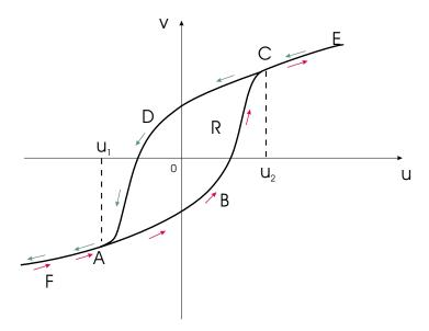
**Figure C-1.** A continuous hysteresis loop for a system whose state is given by the couple (u,v), where u is the input and v is the output (reprinted from *Differential Models of Hysteresis*, 1994, by Augusto Visintin, with permission of Springer-Verlag, GmbH & Co. KG, Heidelberg, Germany).
