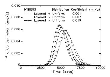
**Figure G-1.** Sensitivity of <sup>99</sup>Tc breakthrough (through the unsaturated zone with a water table at a depth of 6 m) to the distribution coefficients in a layered soil and in a uniform soil using the HYDRUS Model.
