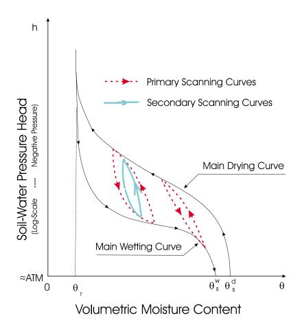
**Figure C-6.** A hypothetical soil-moisture hysteresis loop which is discontinuous for pressure heads near zero, showing the main drying and main wetting curves, and example primary and secondary scanning curves (reprinted from *Subsurface Transport and Fate Processes*, 1993, by R.C. Knox, D.A. Sabatini, and LW. Canter, with permission of CRC Press, Inc., Boca Raton, FL).
