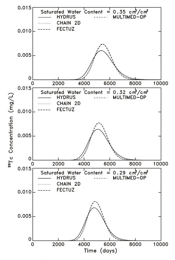
**Figure 7-9.** Sensitivity of  $^{99}$ Tc breakthrough (through the 6m layer) to the saturated water content using the MULTIMED-DP 1.0, FECTUZ, CHAIN 2D and HYDRUS Models, where  $\theta_s = 0.35 \text{ cm}^3/\text{cm}^3$ ,  $0.32 \text{ cm}^3/\text{cm}^3$ , and  $0.29 \text{ cm}^3/\text{cm}^3$ .
