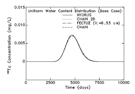
Figure 7-27. Comparison of the  $^{99}$ Tc BTCs for the HYDRUS, CHAIN 2D and CHAIN Models for the base values of the input parameters with the BTC for the FECTUZ Model with the base value of  $D_L = 4.53$  cm replaced by the value  $D_L = 6.53$  cm.
