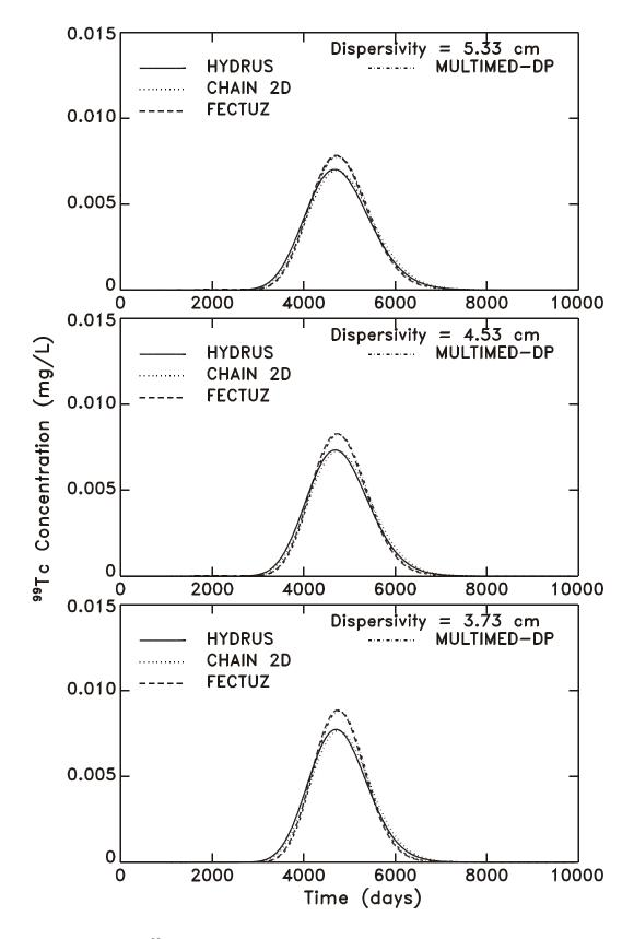
Figure 7-6. Sensitivity of  $^{99}$ Tc breakthrough (through the 6m layer) to the dispersivity using the MULTIMED-DP 1.0, FECTUZ, CHAIN 2D, and HYDRUS Models, where  $D_L = 5.33$  cm, 4.53 cm, and 3.73 cm.
