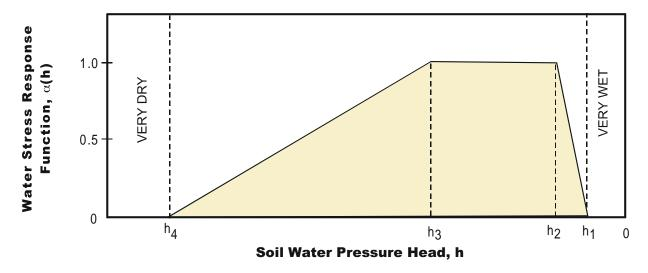
**Figure F-2.** The water stress response function for the Feddes Module of the HYDRUS Code (Šimúnek, et al., 1998).
