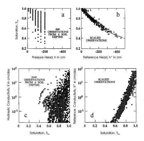
**Figure B-3.** (a) Unscaled observations of  $S_{eo}(h)$ , (b) Scaled observations of  $S_{eo}(h^*)$ , showing the reference relationship as a solid curve, (c) unscaled observations of  $K(S_{eo})$ , and (d) scaled observations of  $K^*(S_{eo})$  (reprinted from *Water Resources Research*, 1977, by A.W. Warrick, G.J. Mullen and D.R. Nielsen with the permission of the American Geophysical Union, Washington, DC).
