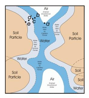
**Figure C-4.** A cross section of a soil pore and the solid soil particles that make up its walls, showing areas drained by the pull of gravity, areas where water is held by capillary forces, and areas where water is held by surface forces (e.g., van der Waals forces) (reprinted from *Soils in Our Environment*, 1995, 7th Ed., by R.W. Miller and R.L. Donahue, with permission of Pearson Education, Inc., Upper Saddle River, NJ).
