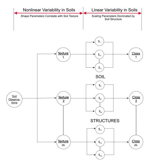
**Figure B-4.** The application of linear scaling to a set of soil-moisture observations, resulting in a set of m similar soil classes. The  $m^{th}$  class of similar soils accounts for the soil structures  $s_{m1}$ ,  $s_{m2}$ , ...,  $s_{mq}$  within the soil textural class m. The number of similar soil classes corresponds to the number of soil textural classes.
