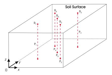
**Figure B-2.** The depiction of a set of vertical soil profiles  $p_1, p_2, ...$  distributed over a field mapping unit, where z represents the local variable within a soil profile and  $R_i$  (i = 1, 2, ...) represent the horizontal vectors in the xy-plane giving the global positioning of the vertical profiles,  $p_1, p_2, ...$
