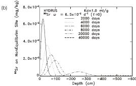
**Figure H-6.** Liquid phase concentration curves (a) and solid phase concentration curves (b) for  $^{90}$ Sr, for various times and for  $\omega = 6.5 \times 10^{-2} d^{-1}$ , where zero depth is the surface and -600 cm is the hypothetical water table.
