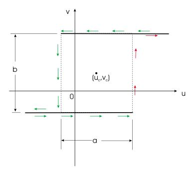
**Figure C-3a.** A relay with hysteresis, or a delayed relay, defined by the parameters (a, b, u<sub>c</sub>, v<sub>c</sub>) with repect to the system defined by states (u,v) (reprinted from *Differential Models of Hysteresis*, 1994, by Augusto Visintin, with permission of Springer-Verlag, GmbH & Co. KG, Heidelberg, Germany).
