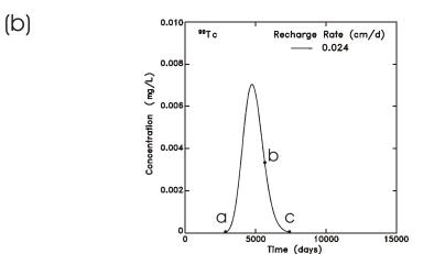
**Figure I-2.** (a) Breakthrough curves of the daughter product, <sup>99</sup>Ru, from the <sup>99</sup>Tc decay using the CHAIN and FECTUZ Models for base case simulation, and (b) the breakthrough curve for <sup>99</sup>Tc. The text will explain a, b, c, d, e and f.
