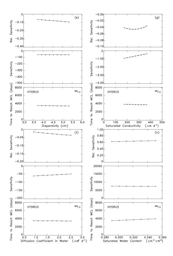
**Figure 6-4.** Sensitivity and relative sensitivity of time to exceed MCL to the system parameters using the HYDRUS Model: (e) dispersivity, (f) diffusion coefficient in water, (g) saturated conductivity, (h) saturated water content.
