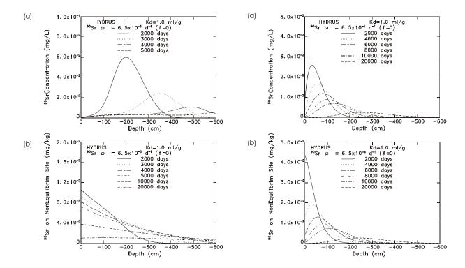
**Figure H-3.** Liquid phase concentration curves (a) and solid phase concentration curves (b) for  $^{90}$ Sr, for various times and for  $\omega = 6.5 \times 10^{-5} \text{d}^{-1}$ , where zero depth is the surface and -600 cm is the hypothetical water table.
