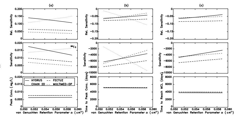
Figure 7-23. Sensitivity and relative sensitivity of (a) peak concentration at the depth of 6m, (b) time to reach peak concentration at the depth of 6m, and (c) time to exceed MCL at the receptor well to the van Genuchten retention parameter α using the MULTIMED-DP 1.0, FECTUZ, CHAIN 2D, and HYDRUS Models.
