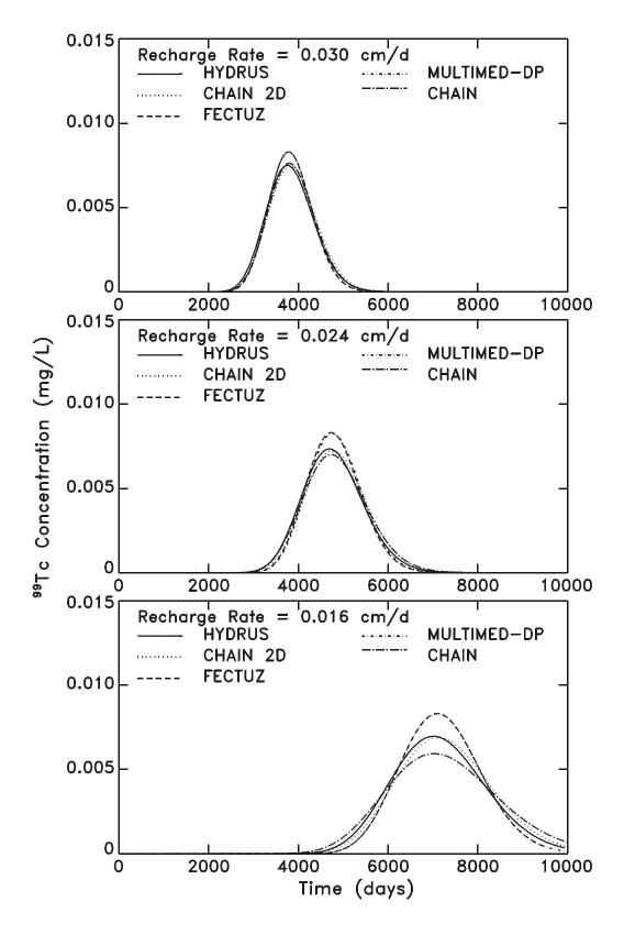
Figure 7-2. Sensitivity of  $^{99}$ Tc breakthrough (through the 6m layer) to the recharge rate using the CHAIN, MULTIMED-DP 1.0, FECTUZ, CHAIN 2D, and HYDRUS Models, where q = 0.030 cm/d, 0.024 cm/d, and 0.016 cm/d.
