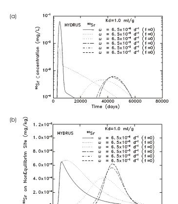
Figure H-2. (a) Breakthrough curves for the liquid phase concentration at the 6 m level. (b) Concentration curves for the nonequilibrium solid phase at the 6 m depth. Curves for  $\omega = 6.5 \times 10^{-2} \text{d}^{-1}$  and  $6.5 \times 10^{-2} \text{d}^{-1}$ 10<sup>-1</sup>d<sup>-1</sup> are basically the same for both (a) and (b).
