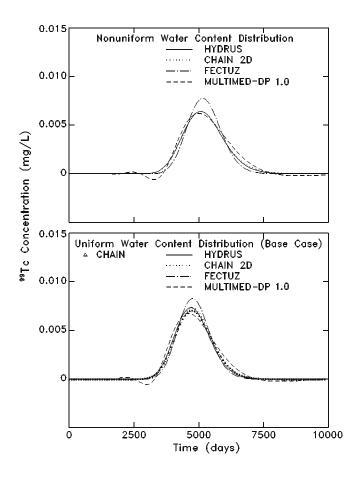
Figure E-2. Comparison of the breakthrough curves predicted by the CHAIN, HYDRUS, CHAIN 2D, FECTUZ, and MULTIIMED-DP 1.0 Models for the base case given in Section 6. The top curves are for a nonuniform water content and the bottom curves are for  $\theta = 0.16$  throughout the soil column. There are no CHAIN results in the top graph because  $\theta$  can only be constant in this model.
