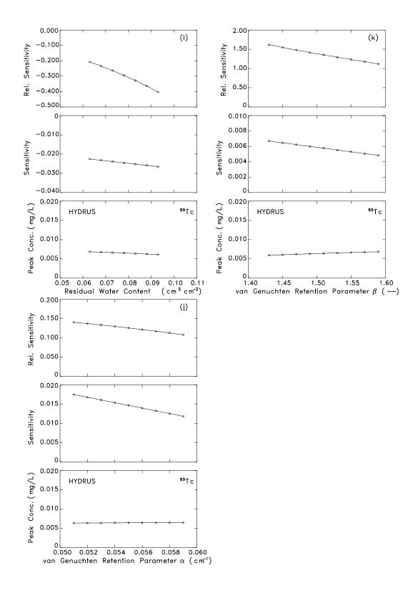
**Figure 6-2.** Sensitivity and relative sensitivity of peak concentrations at the depth of 6m to the system parameters using the HYDRUS Model: (i) residual water content, (j) van Genuchten retention parameter  $\alpha$ , (k) van Genuchten retention parameter  $\beta$ .
