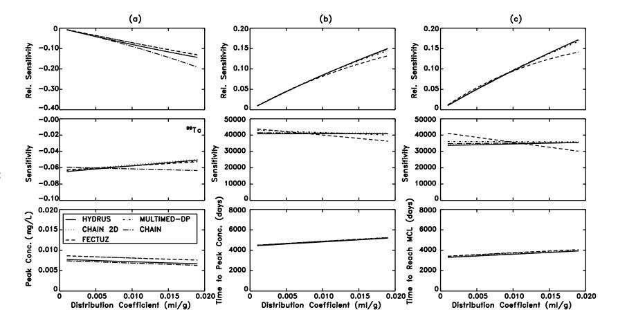
**Figure 7-13.** Sensitivity and relative sensitivity of (a) peak concentration at the depth of 6m, (b) time to reach peak concentration at the depth of 6m, and (c) time to exceed MCL at the receptor well to the distribution coefficient using the CHAIN, MULTIMED-DP 1.0, FECTUZ, CHAIN 2D and HYDRUS Models.
