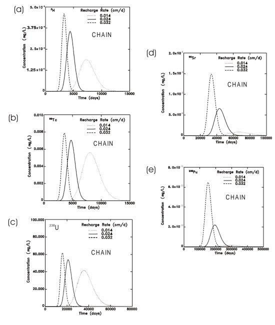
**Figure I-3.** Sensitivity of radionuclide transport through the unsaturated zone to recharge rate (q) using the CHAIN Model: (a) Tritium <sup>3</sup>H; (b) Technetium <sup>99</sup>Tc; (c) Uranium <sup>238</sup>U; (d) Strontium <sup>90</sup>Sr; and (e) Plutonium <sup>238</sup>Pu.
