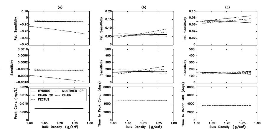
Figure 7-16. Sensitivity and relative sensitivity of (a) peak concentration at the depth of 6m, (b) time to reach peak concentration at the depth of 6m, and (c) time to exceed MCL at the receptor well to the bulk density using the CHAIN, MULTIMED-DP 1.0, FECTUZ, CHAIN 2D and HYDRUS Models.
