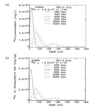
**Figure H-5.** Liquid phase concentration curves (a) and solid phase concentration curves (b) for  $^{90}$ Sr, for various times and for  $\omega$  = 6.5 x  $10^{-3}$ d<sup>-1</sup>, where zero depth is the surface and -600 cm is the hypothetical water table.
