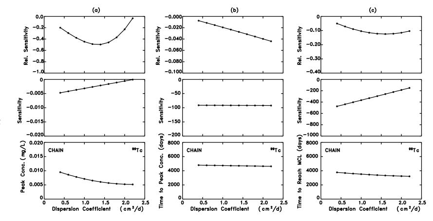
**Figure 7-17.** Sensitivity and relative sensitivity of (a) peak concentration at the depth of 6m, (b) time to reach peak concentration at the depth of 6m, and (c) time to exceed MCL at the receptor well to the dispersion coefficient using the CHAIN Model.
